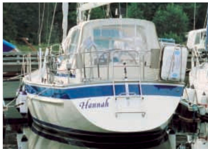
This is the standard reverse transom with a folding ladder for access to the water.
