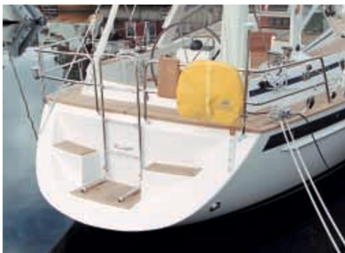
The integrated bathing platform of this standard reverse transom gives easy access to the water for swimming and bathing.
