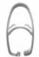
Extra wide sail slot for vertical battens.
